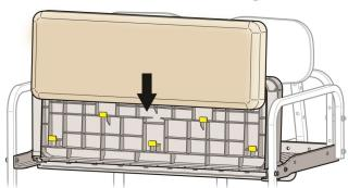
Fasten the handle to the seat platform using (2) 6mm x 20 Phillips Head Countersunk Screws (Bag #5). Hand tighten to lock the seat bottom into place.
