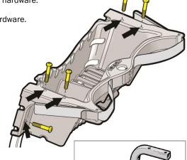
Remove both seat back support brackets and rubber boots. The brackets are attached to the frame, under the body.
