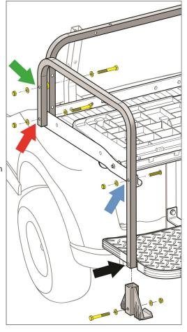
Install the rear seat back brackets to the rear seat back using (4) 6mm x 25 Hex Head Bolts, (4) 6mm Lock Washers and (4) 6mm Flat Washers (Bag #5). Hand tighten.
