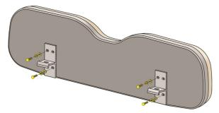
17. Install the rear seat back assembly to the rear seat back support frame using (2) 10mm x 45 Hex Head Bolts, (4) 10mm Flat Washers and (2) 10mm Nylock Nuts (Bag #5).
