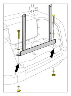
6. Loosely install the seat platform and seat platform support bracket to the front seat back support brackets using (2) 10mm x 35 Hex Head Bolts, (4) Flat Washers and (2) Nylock Nuts (Bag #2).
