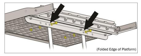
8. Loosely fasten the footplate to the vertical support bracket using (2) 10mm x 35 Hex Head Bolts, (4) Flat Washers and (2) Nylock Nuts (Bag #3).
